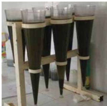
Figure 5: Imhoff cones being used in analyses of sludge volume index (source: SANDEC).
