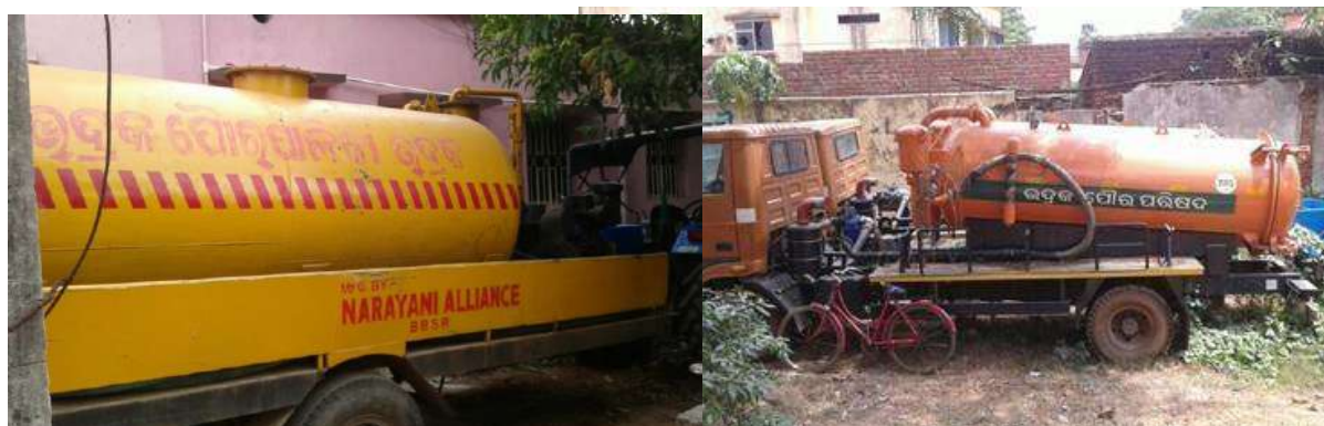
Figure 4-8: -Old (left) and new cesspool emptying trucks (right) of Bhadrak Municipality
